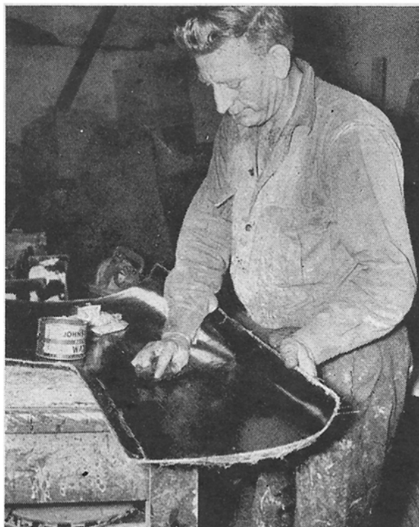
Wax is applied to the mould before the fibreglass and resin are laid in, otherwise the body would adhere to the mould.
